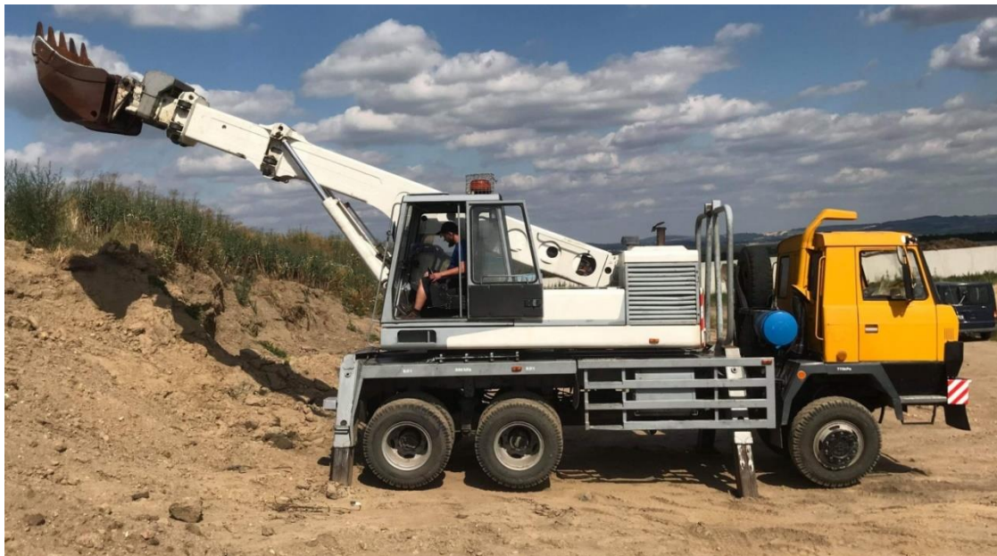
Fig. 1 Telescopic excavator UDS 214 on a Tatra 815 chassis during practical testing of working cycle time
