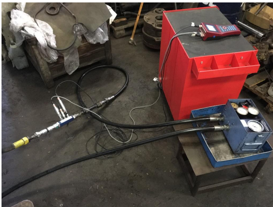
Fig. 4 Connection of the analog meter OTC H50 and the digital meter from Hydrotechnik into the examined hydraulic circuit (measurement at the beginning of the hydraulic circuit)
